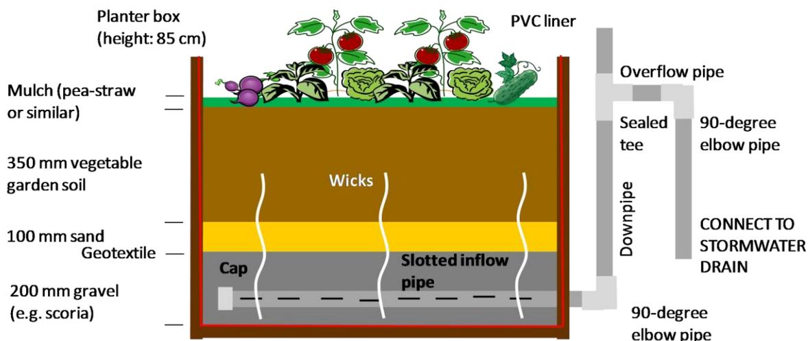
**Figure 2.26: Schematic diagram showing how wicks could be added to a sub-irrigated vegetable raingarden to promote capillary rise, and a simpler overflow design (replacing the pits in this study) that would allow a higher water level.**
