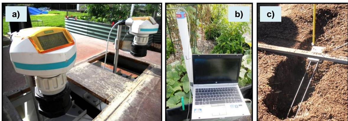
**Figure 2.10: Monitoring equipment: a) The two ultrasonic level monitors (attached to the flumes) for measuring inflow to the raingardens, b) Data being downloaded from the Odyssey capacitance depth logger (in its PVC pipe) in the Lined raingarden, and c) a CS616 Water Content Reflectometer being installed in the soil.**
