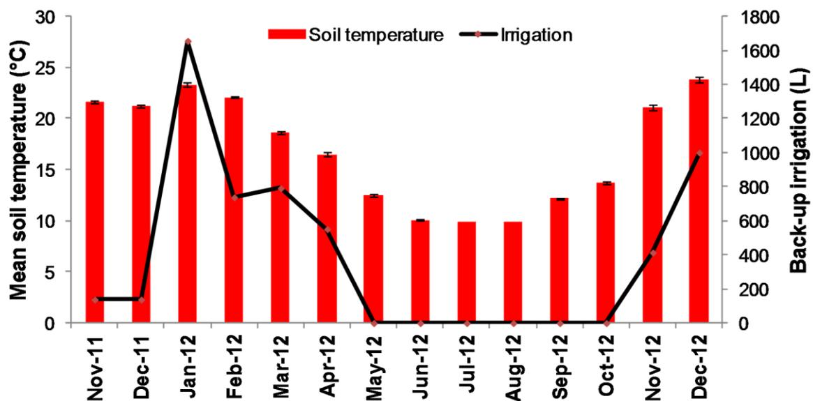
Figure 2.16: Irrigation requirements for the Unlined raingarden under the deficit irrigation regime (black line), in relation to mean ( $\pm$  SE) soil temperature for each month (red bars). There is no soil temperature data for 2013.
