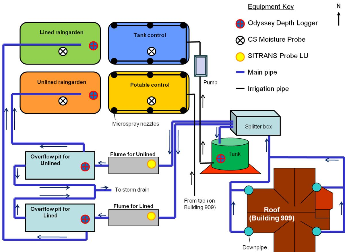
**Figure 2.6: Schematic diagram of the plumbing system, including monitoring equipment. For clarity, the drip irrigation system in the Unlined raingarden (connected to the tank) is not shown. Arrows indicate the direction of water flow through the system. The components of the system are not to scale.**
