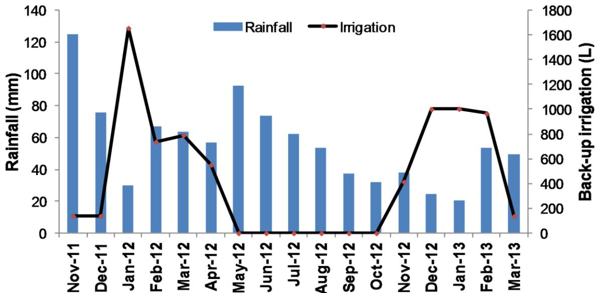
Figure 2.15: Irrigation requirements for the Unlined raingarden under the deficit irrigation regime (black line), in relation to monthly rainfall totals (blue bars).
