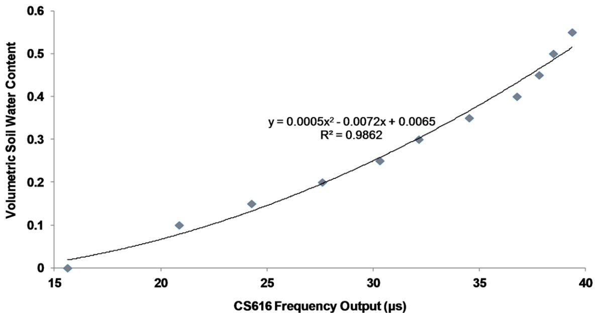
**Figure AE-2: Calibration of the CS616 soil moisture probe for the field trial soil; volumetric water content and corresponding CS616 output periods.**
