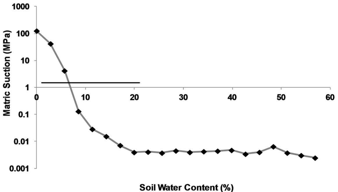
**Figure AC-2: Matric suction plotted against soil water content for the field trial soil. The horizontal line represents the permanent wilting point.**
