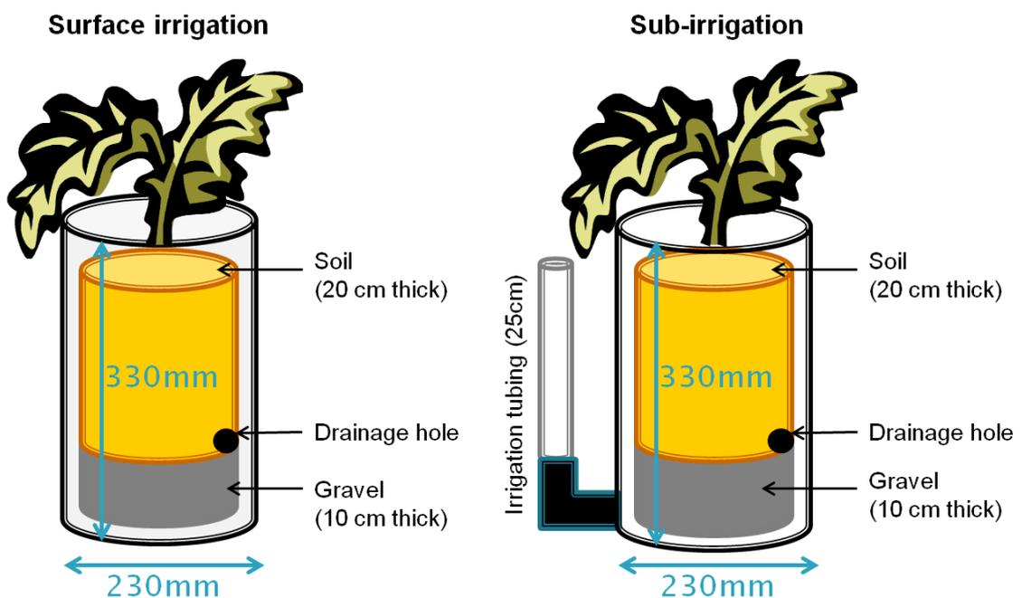
**Figure 3.1: Design of the surface-irrigated pots (left) and sub-irrigated pots (right).**
