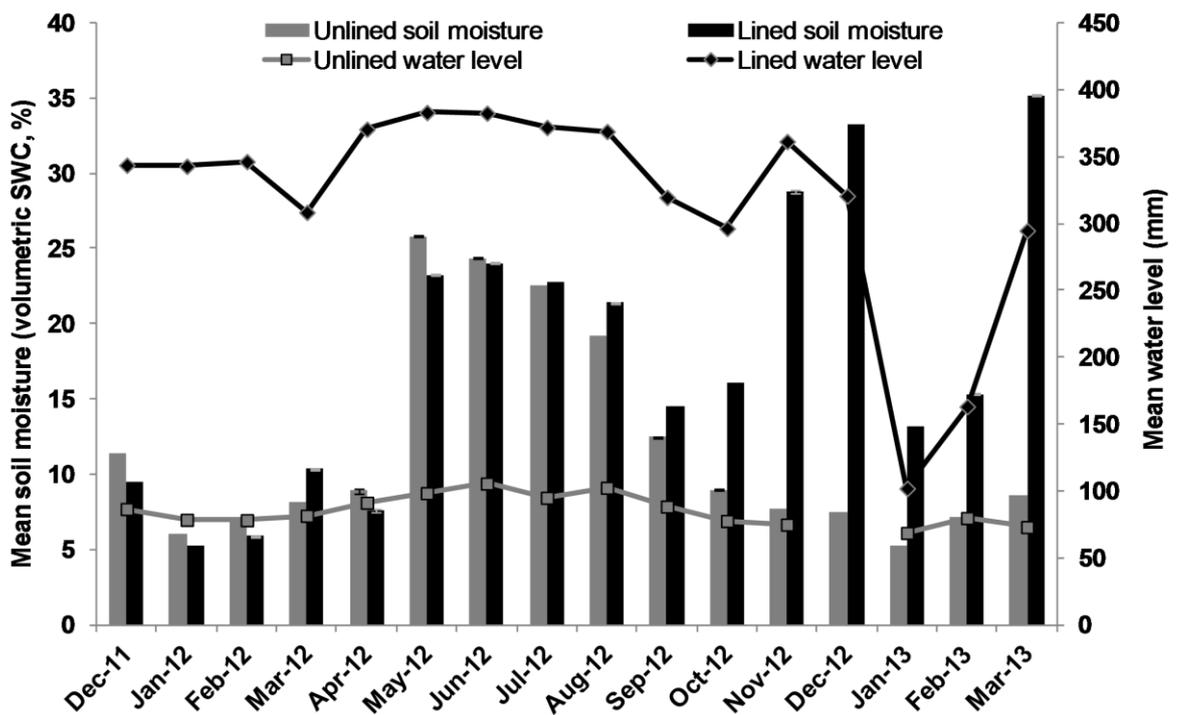
Figure 2.14: Mean ( $\pm$  SE) soil moisture in the two raingardens, Unlined (grey bars) and Lined (black bars), and the relationship with mean ( $\pm$  SE) water level for each month. For the Unlined raingarden, there is no water level data for December 2012.
