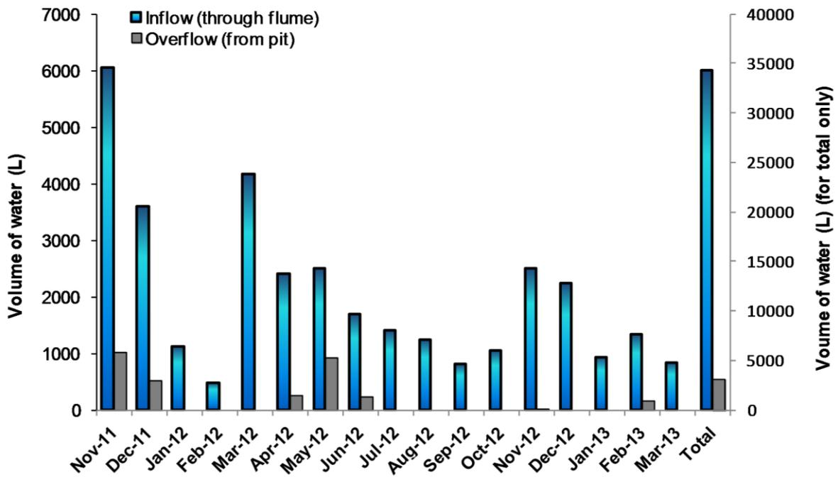
Figure 2.20: Total volume of inflow (through the flume) in comparison to the total volume of overflow (to the stormwater drain) for the Unlined raingarden.
