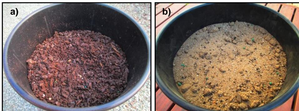
**Figure 3.2: Samples of the potting mix (a) and the loamy sand (b).**
