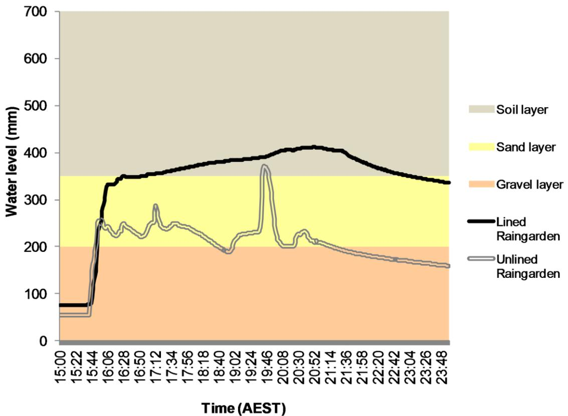
**Figure 2.17: Water level in the two raingardens between 3 pm and 11.59 pm (AEST) on 28<sup>th</sup> September 2011, following heavy rainfall. The approximate boundaries of the filter/growing media layers are presented for comparison.**
