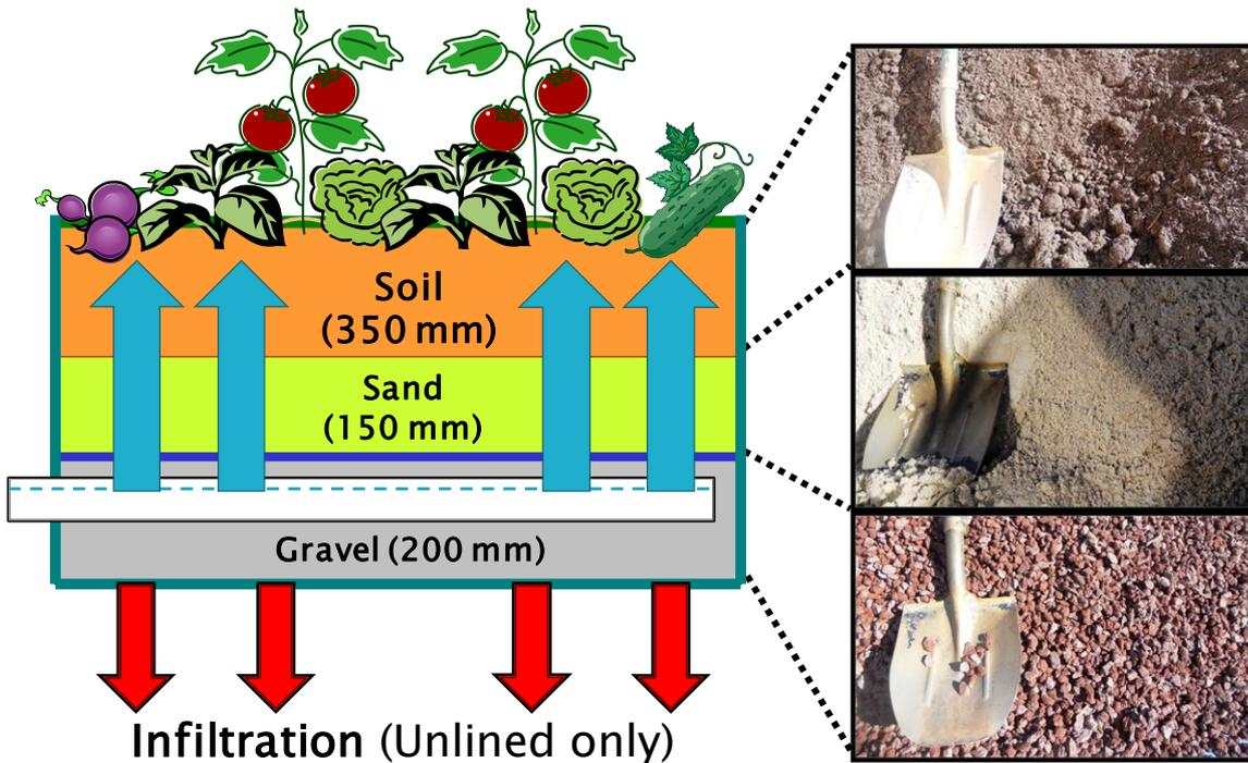
Figure 2.4: Design of the two raingardens. Water enters via a slotted pipe in the gravel layer (bottom) and moves upwards, through a layer of sand (middle) and into a layer of soil (top). Blue arrows indicate upwards movement of water via capillary rise. Red arrows indicate infiltration into the underlying soil.
