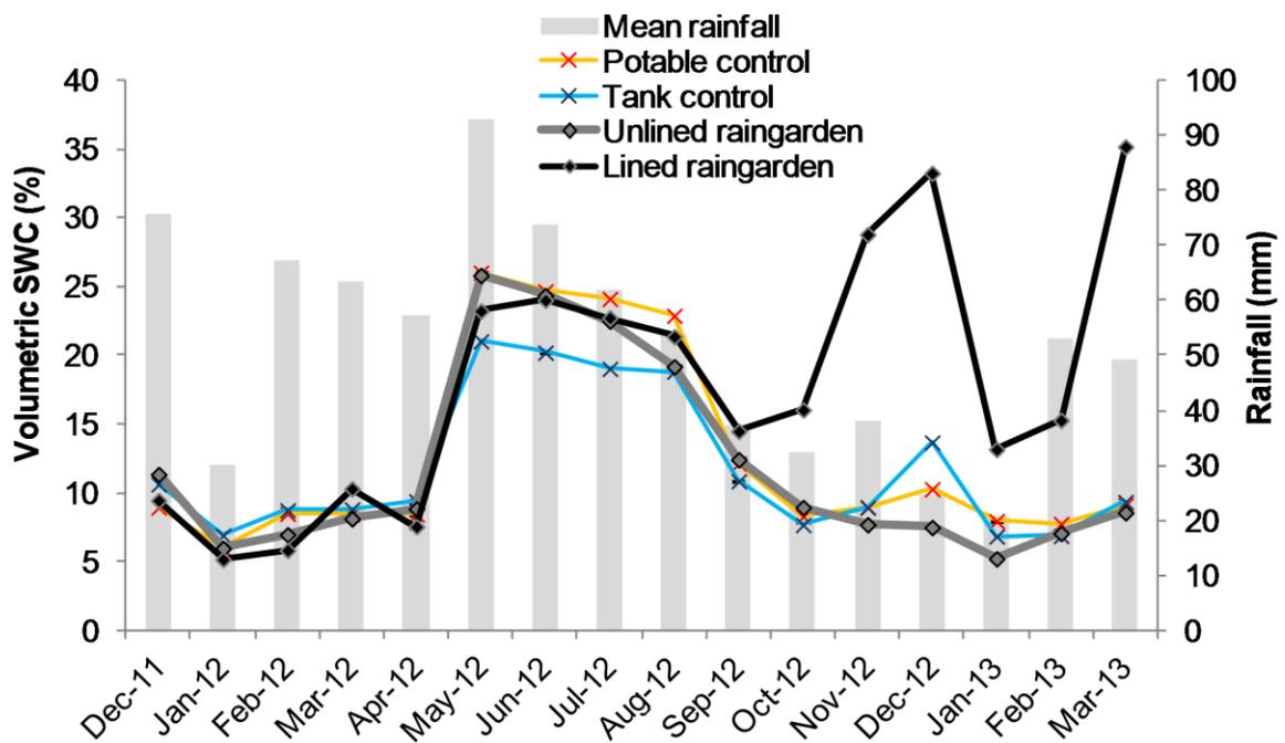
**Figure 2.12: Mean soil moisture ( $\pm$  SE) in the four garden beds in each month of the monitoring period (except November 2012, when probes were not calibrated), with rainfall totals for comparison. Further details are presented in Appendix G. CS616 probes are checked in standard media to ensure accuracy of  $\pm$  2% volumetric water content (Campbell Scientific Inc., 2002).**
