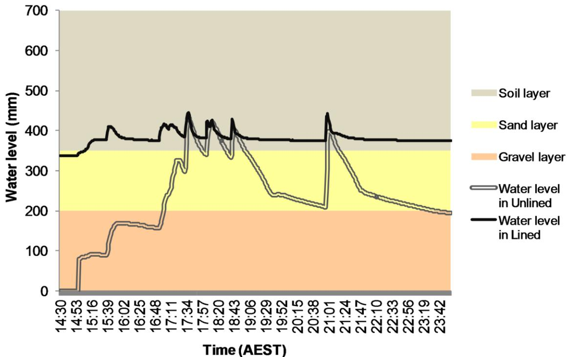
**Figure 2.23: Water level in the two raingardens between 2.30 pm and 11.59 pm (AEST) on 25<sup>th</sup> December 2011. The approximate boundaries of the filter/growing media layers are presented for comparison.**
