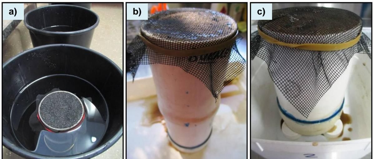
**Figure AB-1: The main stages of the AFP procedure: a) Soaking the apparatus, b) draining the apparatus (both sections, viewed from above), and c) draining the bottom section only.**
