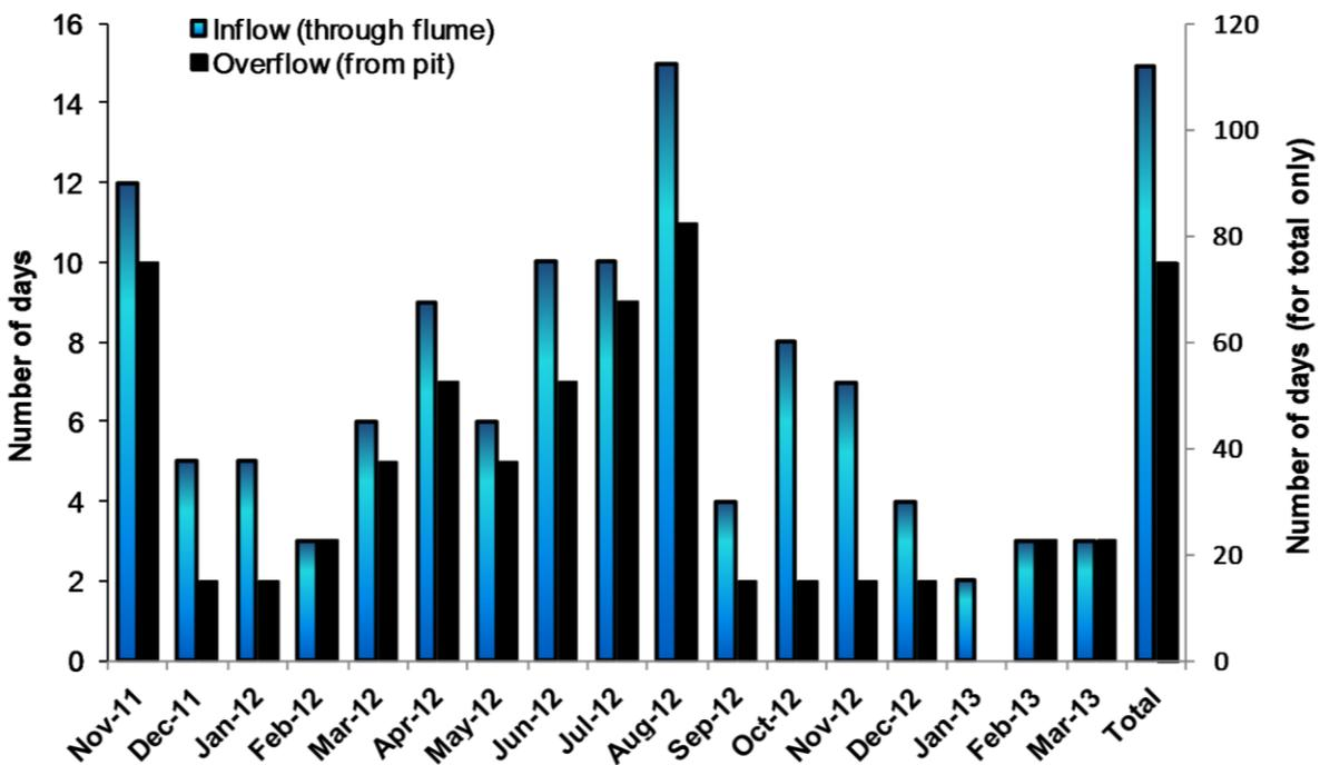
Figure 2.19: Number of days per month of inflow ( $> 1 \text{ L m}^{-1}$ ) to the Lined raingarden compared to the number of days of overflow.
