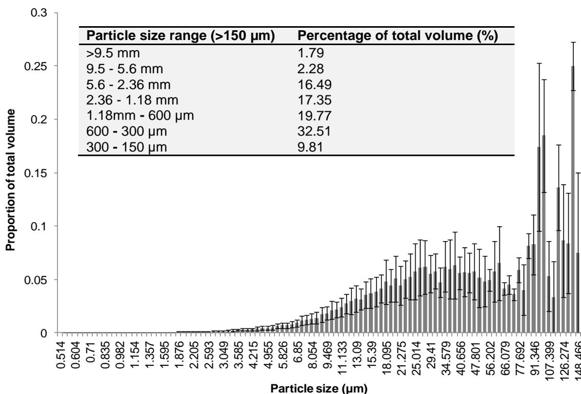
Figure AA-1: Particle size distribution in a <150 μm sample of the field trial (“Five Way”) soil, measured using an AccuSizer Autodiluter AD. Error bars represent standard error (n = 3). INSET: Table showing particle size distribution for size ranges >150 μm, measured by sieving and weighing (Australian Standards AS 1289.3.6.1 2009). All measurements were made by Minna Tom (Monash University).
