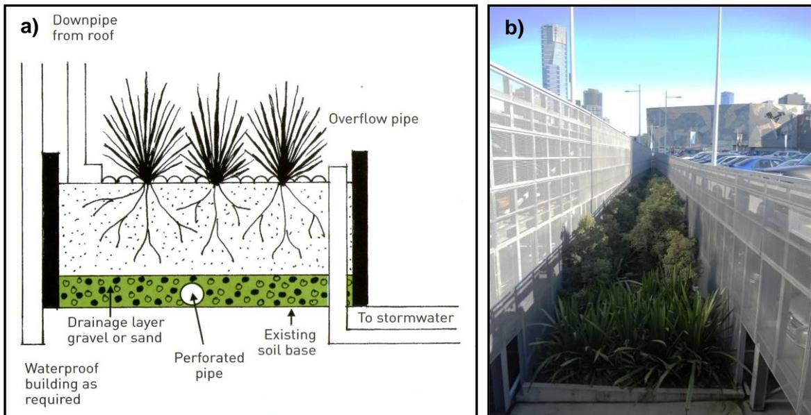
**Figure 1.3: a) Schematic section through a typical raingarden (McQuire, 2008), and b) A large raingarden at Federation Square in Melbourne's city centre, adjacent to the Yarra River.**
