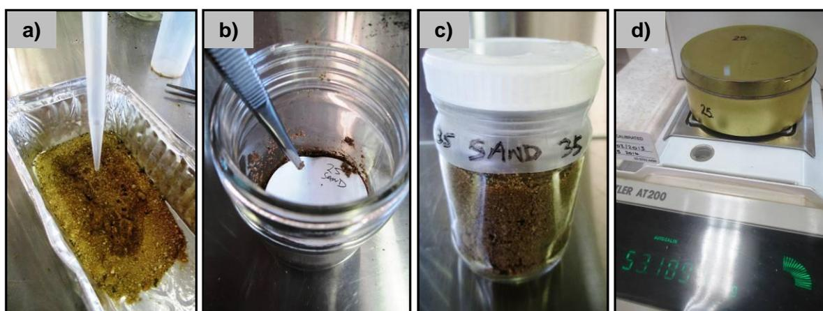
**Figure AC-1: Method for measuring soil matric potential: a) Adding water to the soil using a pipette, b) Placing filter paper over the bottom portion of soil, c) A fully-sealed jar containing the two portions of soil, separated by the filter paper, and d) Measuring the weight of a tin, containing the oven-dried filter paper.**
