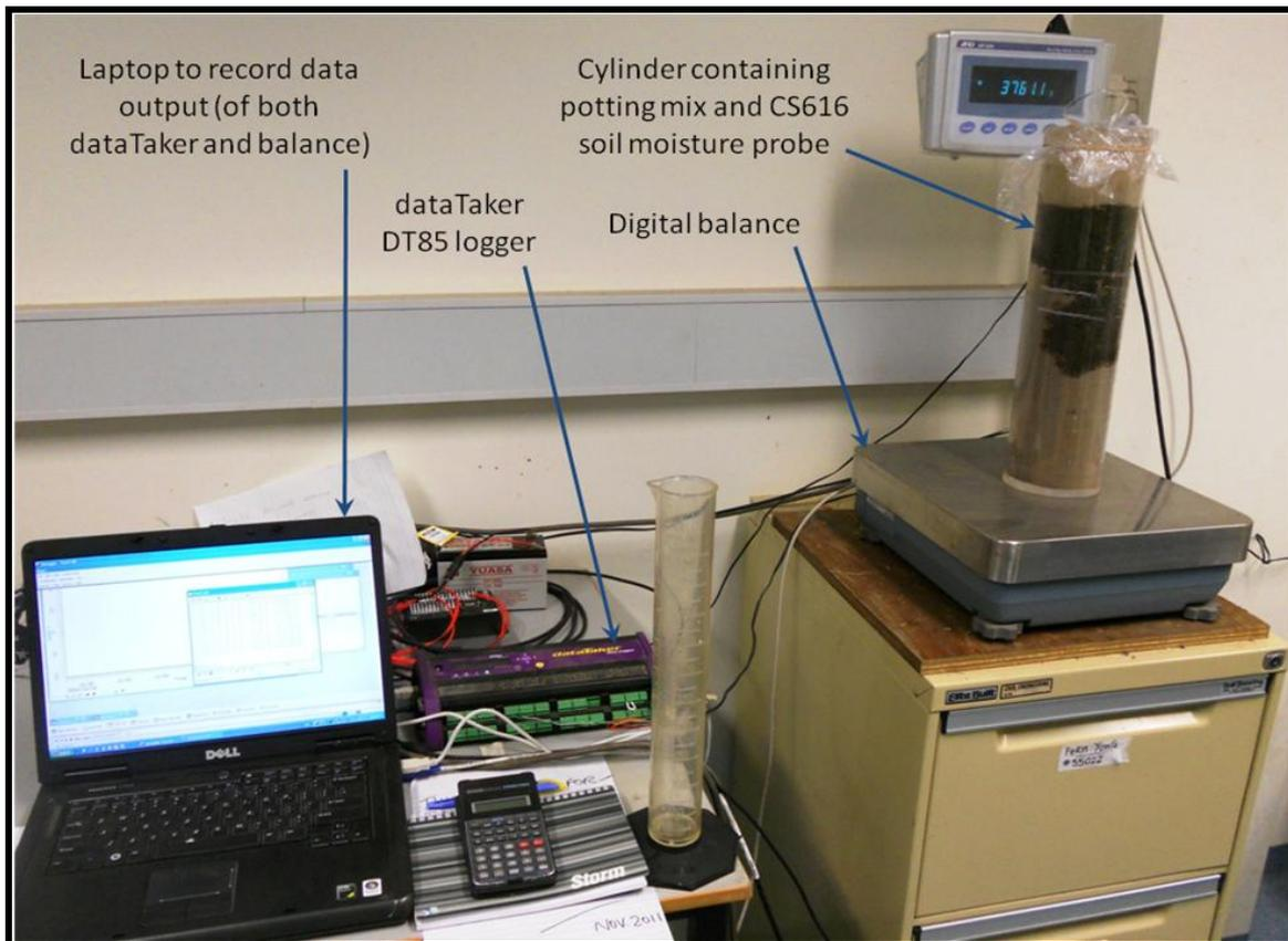
**Figure AE-1: Laboratory setup for calibration of the CS616 soil moisture probe.**
