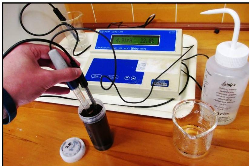
Figure AD-1: Measuring the pH of a potting mix supernatant.
