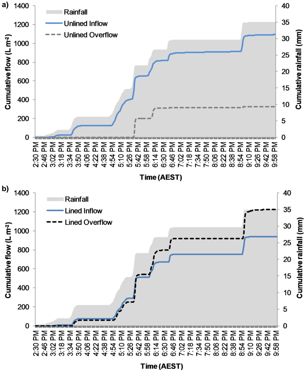
Figure 2.22: Cumulative inflow and overflow hydrographs for the Unlined (a) and Lined (b) raingardens for the period 2.30 pm to 10 pm (AEST) on 25<sup>th</sup> December 2011, with total rainfall (cumulative) at the site for comparison.
