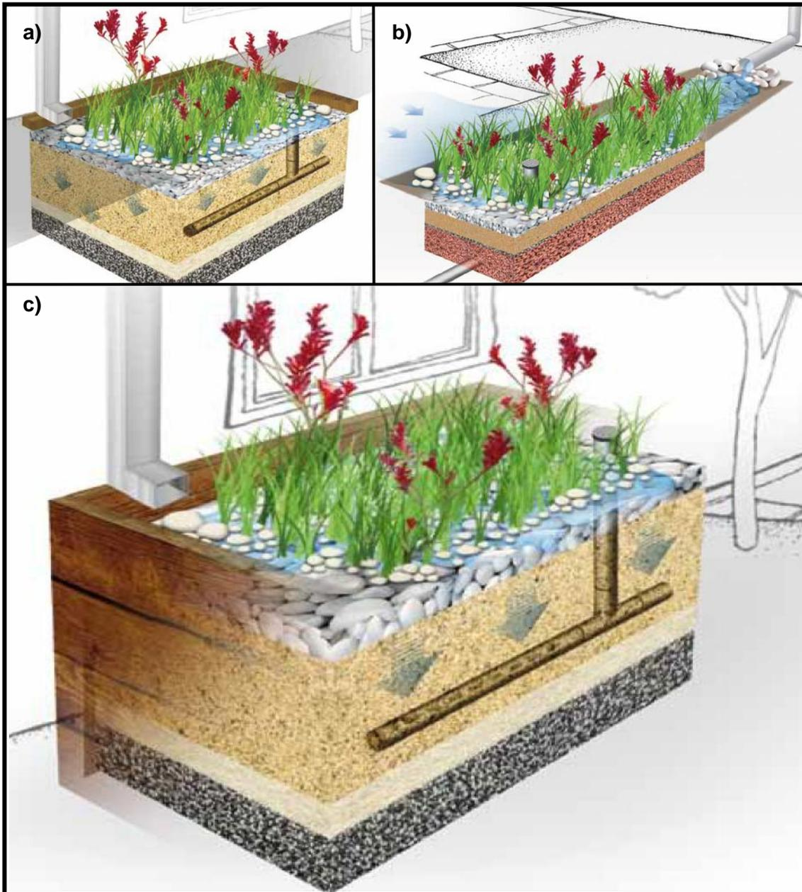
**Figure 1.4: a) In-ground lined raingarden (Melbourne Water, 2010a), b) Infiltration raingarden (Melbourne Water, 2010c), and c) Planter-box lined raingarden (Melbourne Water, 2010b).**
