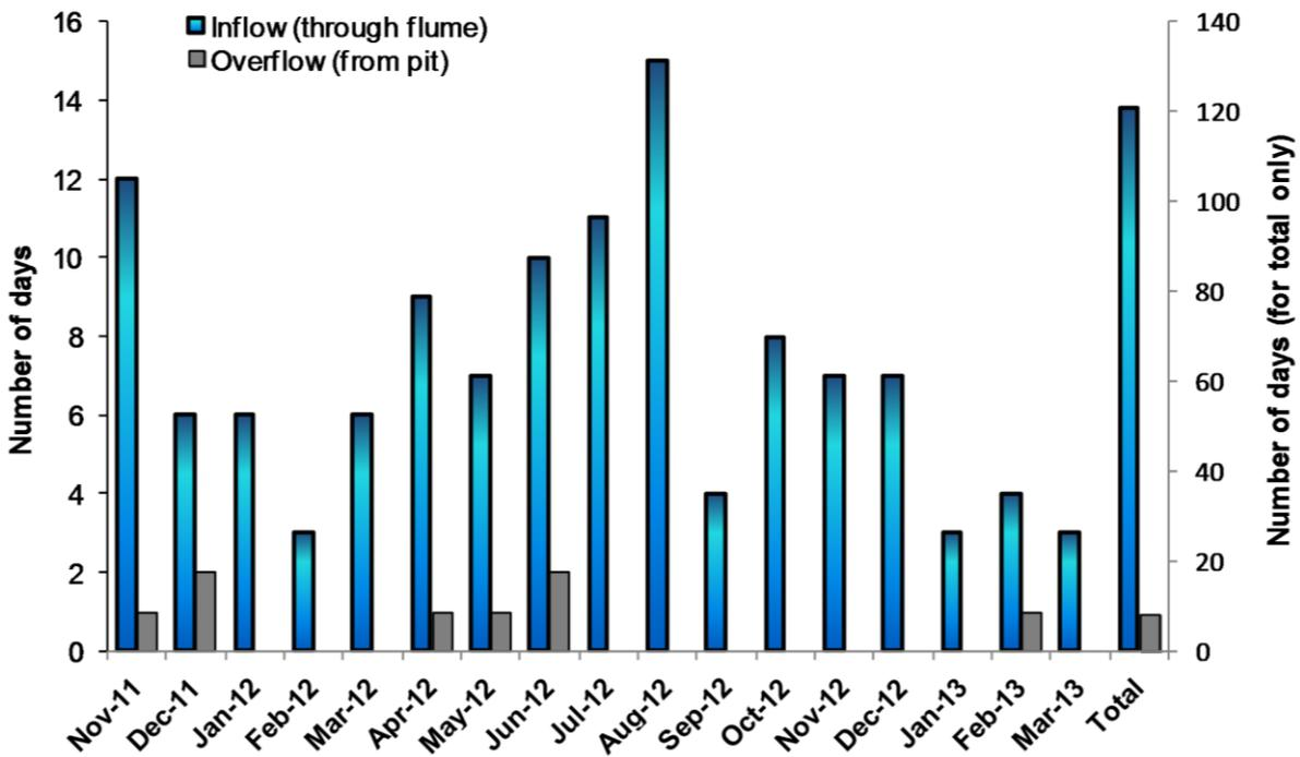
Figure 2.18: Number of days per month of inflow ( $> 1 \text{ L m}^{-1}$ ) to the Unlined raingarden compared to the number of days of overflow.
