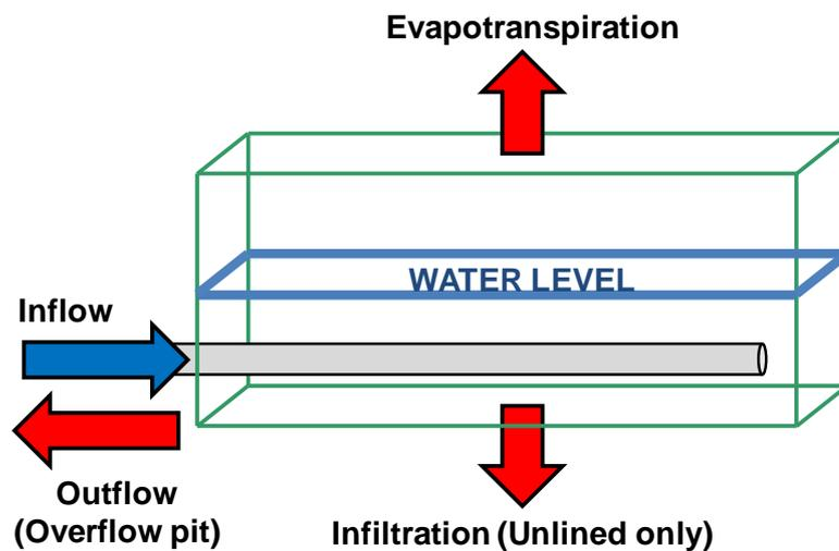
Figure 2.11: Principles for evaluating the water balance of the raingardens.
