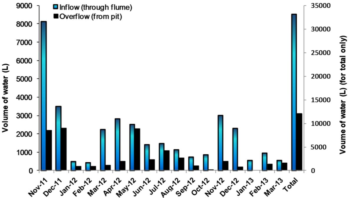
Figure 2.21: Total volume of inflow (through the flume) in comparison to the total volume of overflow (to the stormwater drain) for the Lined raingarden.
